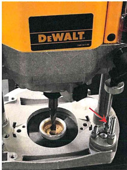
Short stop/deepest cut (42 mm) with stop bar pushed in as shown in Fig. 12.
