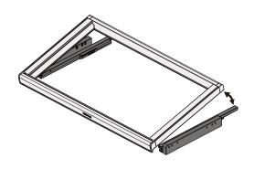
2.2 Position the rear section of the front of the frame onto the front of the slides, then lower the back of the frame until it locks completely.
